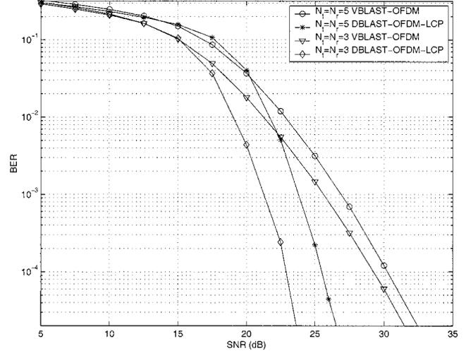
Fig. 2. DBLAST-OFDM-LCP versus VBLAST-OFDM.
