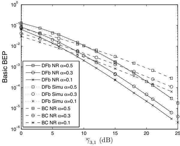
Fig. 5. BEP comparison for BC using 2/4-PAM vs. 2-tier CBC using 4/16-QAM with DFb.
