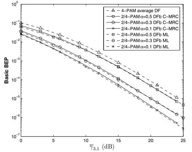
Fig. 6. BEP comparison for 2-tier CBC using 2/4-PAM with DFb (C-MRC and ML) vs. 4-PAM with DF.
