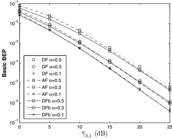
Fig. 7. BEP comparison for 2-tier CBC using 2/4-PAM with DFb vs. DF vs. AF.
