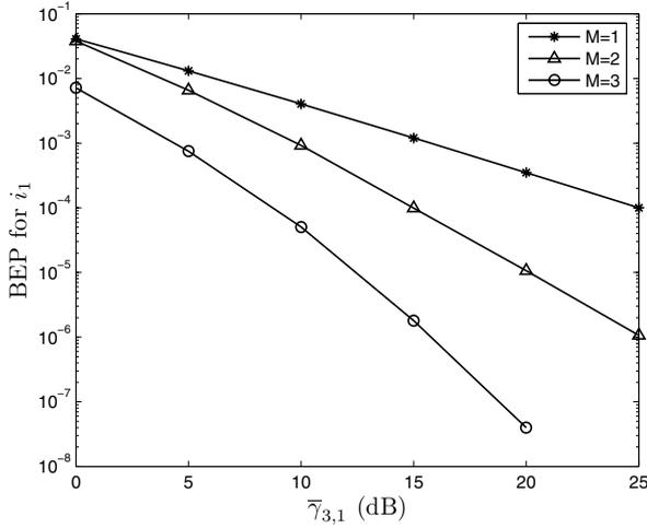
Fig. 10. BEP comparison for bit  $i_1$  at  $T_1$  in  $M$ -tier CBC using 2/4-PAM and DFb with  $\alpha = 0.3$ .
