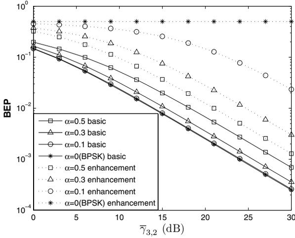
Fig. 4. BEP comparison for bits  $i_1$  and  $i_2$  at  $T_2$  (point-to-point link).
