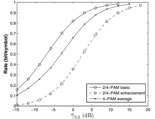
Fig. 9. Achievable rate comparison of both basic and enhancement information at  $T_2$  for BC using 2/4-PAM with  $\alpha = 0.3$  vs. 4-PAM with average rate.
