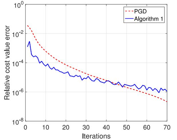
Fig. 5. Cost convergence for Alg. 1 and PGD.
