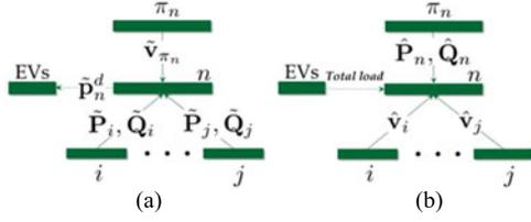
Fig. 3. Information exchange in the ADMM steps for bus  $n$ . (a) First step of ADMM. (b) Second step of ADMM.
