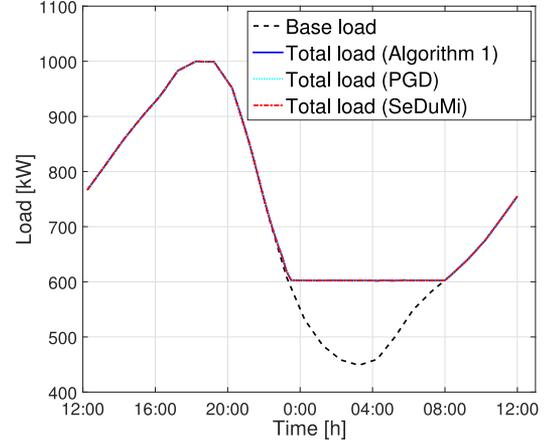
Fig. 4. Load curves after optimal charging of 59 EVs.
