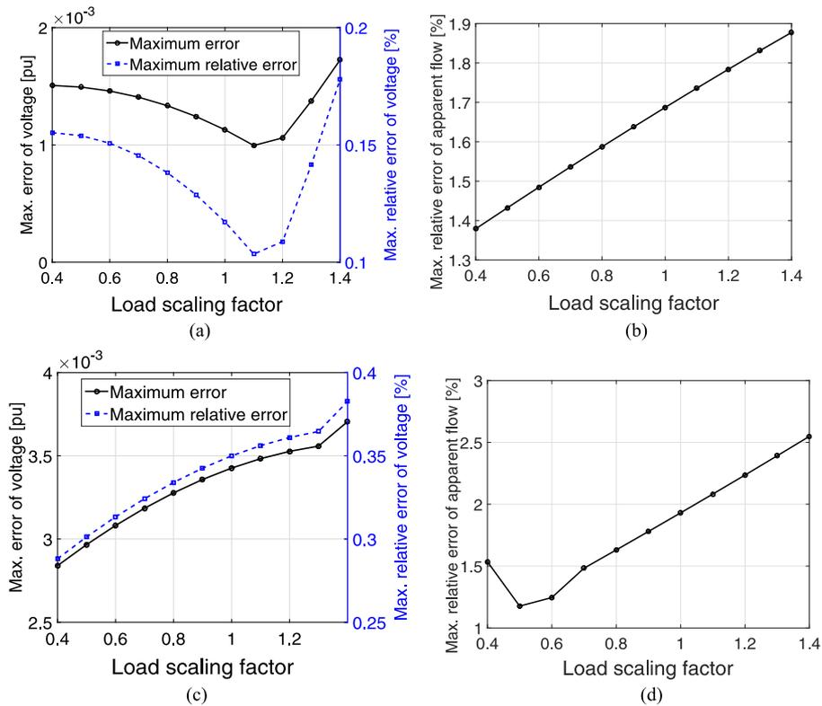
Fig. 10. Approximation error between the full ac and the linearized power flow models for increasing loading factor. (a) Voltages in 13-bus feeder. (b) Apparent flows in 13-bus feeder. (c) Voltages in 123-bus feeder. (d) Apparent flows in 123-bus feeder.
