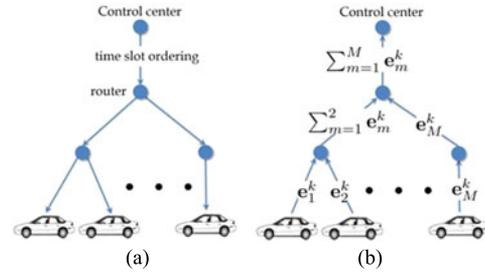
Fig. 1. Information exchange for Algorithm 1 at iteration  $k$ . (a) Control center broadcasts time slot pricing ordering (from cheapest to most expensive) to EV controllers. (b) Summations of charging profiles are transmitted to charging control center.
