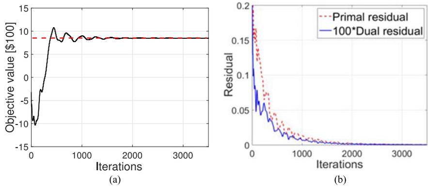
Fig. 9. Convergence performance for the IEEE 123-bus feeder. (a) Objective value convergence. (b) Primal/dual residual convergence.
