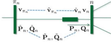
Fig. 2. Consensus and duplicate variables in the ADMM scheme. Variables connected by blue dotted lines are constrained to be equal.
