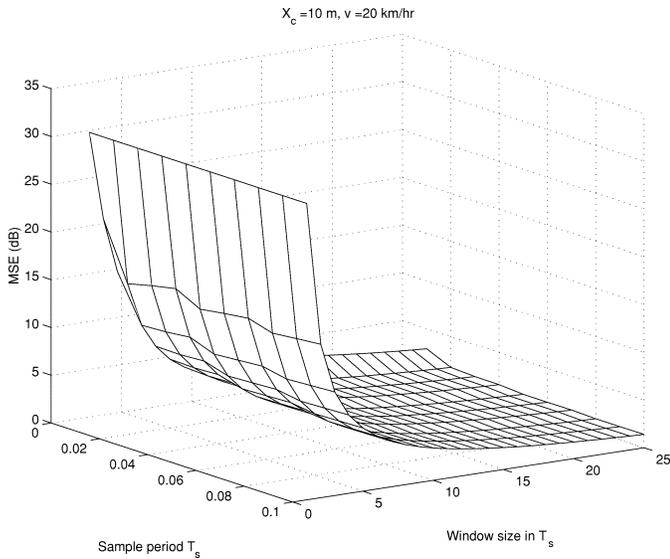
Fig. 1. MSE versus  $T_s$  and window size in  $T_s$ .
