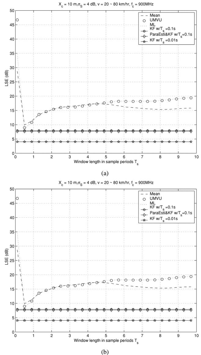
Fig. 7. KF without parameter estimation versus KF with parameter estimation. (a) KF with large to moderately small  $T_s$ . (b) KF with very small  $T_s$ .
