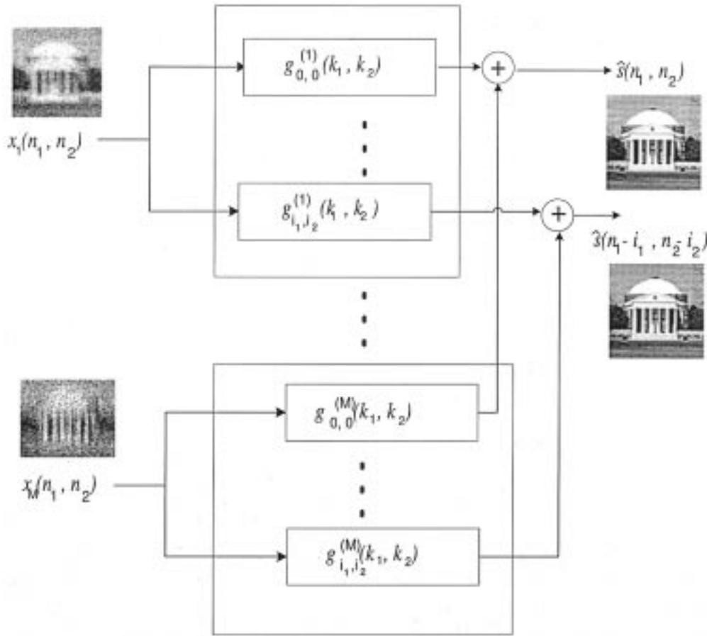
Fig. 3. Multiple-lag restoration filters.
