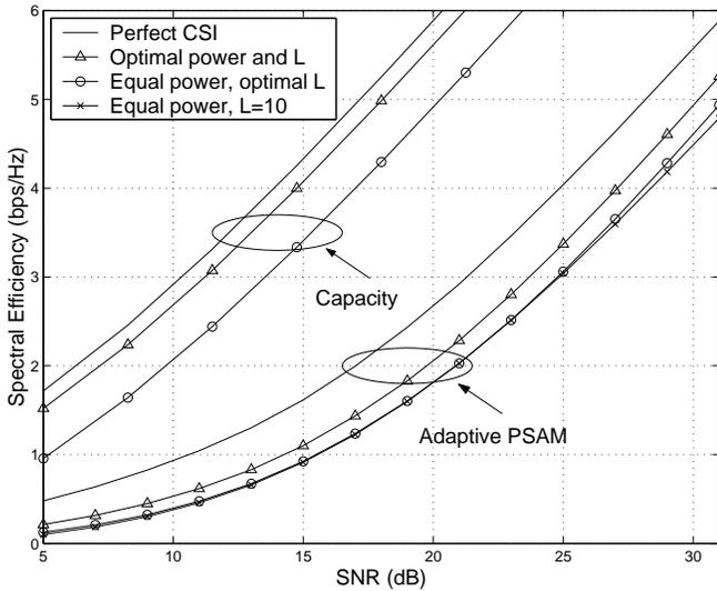
Figure 4: Spectral efficiency of constant power adaptive modulation
