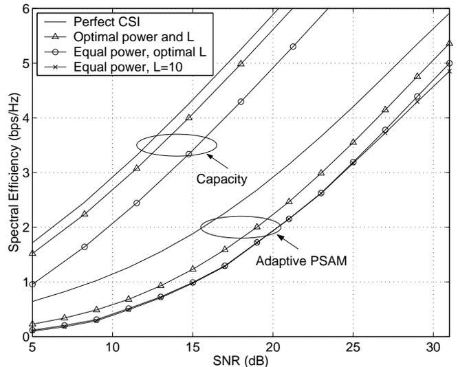
Figure 5: Spectral efficiency of discrete power adaptive modulation
