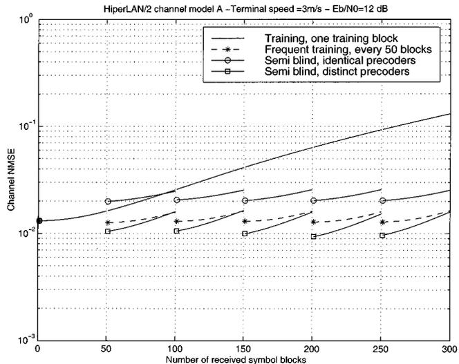
Fig. 4. Channel NMSE along the data burst  $N_p = 4$ .
