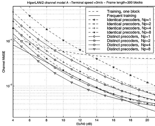
Fig. 6. Channel NMSE versus SNR (slowly time-varying channels).
