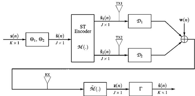
Fig. 1. Block precoded ST-OFDM transceiver model.
