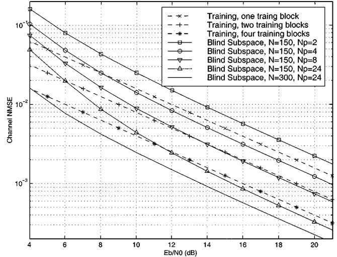
Fig. 2. Training versus blind subspace based channel estimation (static channels).
