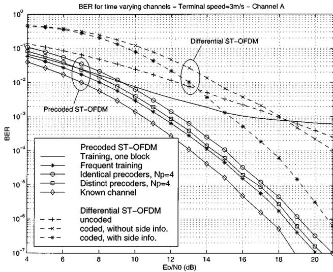
Fig. 9. BER comparisons  $v = 3$  m/s,  $W = 100$  blocks.
