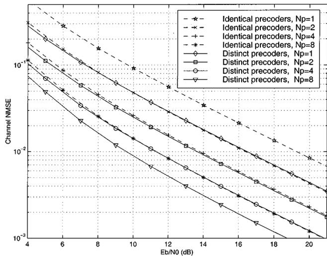
Fig. 3. Identical versus distinct precoders (static channels).
