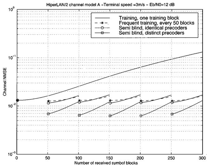
Fig. 5. Channel NMSE along the data burst  $N_p = 8$ .
