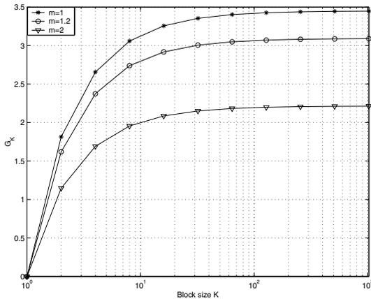
Fig. 2. The SNR gain of UP-OFDMA over OFDMA
