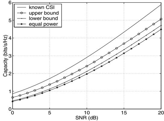
Fig. 1. Channel capacity bounds vs. SNR (Low-pass model)
