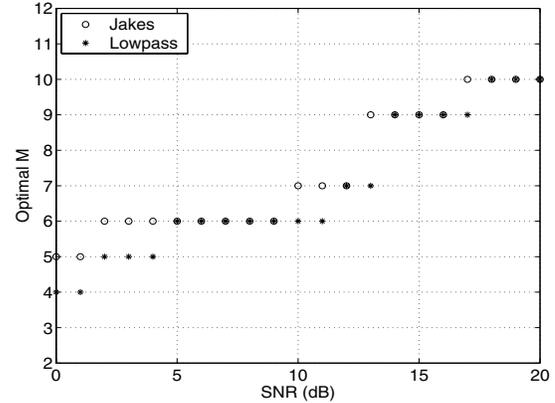
Fig. 3. Optimal pilot spacing vs. SNR (equi-powered PSAM)
