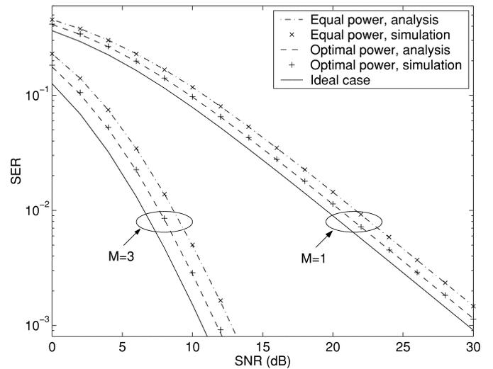
Fig. 3. SER versus SNR (MMSE channel estimation).
