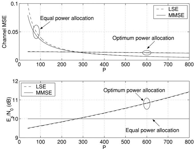
Fig. 5. Channel MSE and transmitted SNR per information symbol versus number of pilot symbols.
