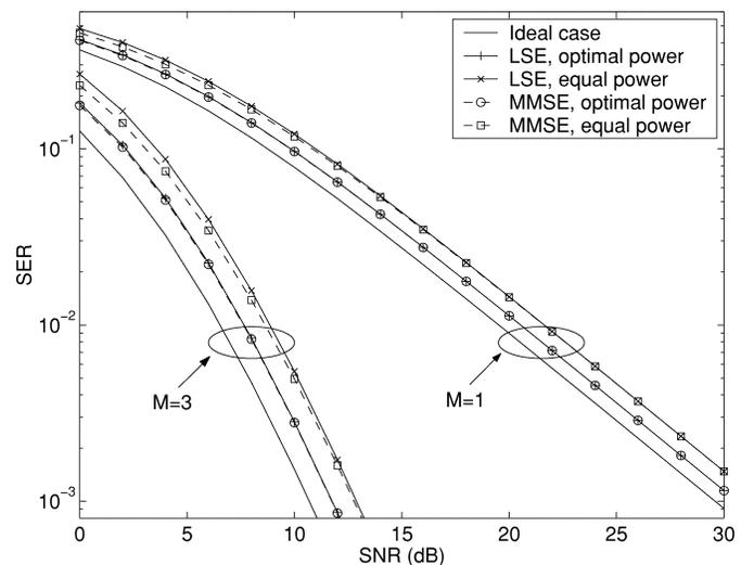
Fig. 4. SER comparison between LSE and MMSE channel estimation.
