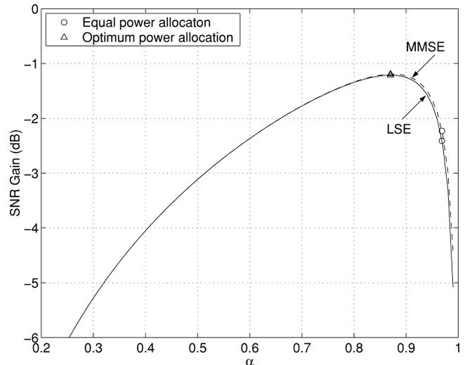
Fig. 6. Effect of power allocation on performance loss.
