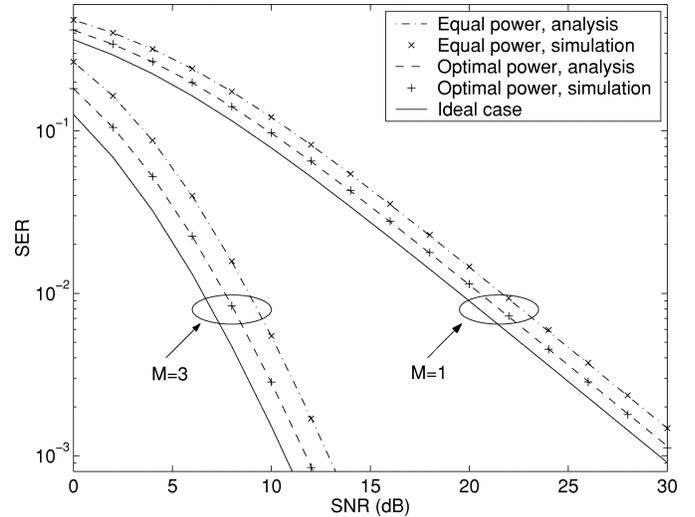
Fig. 2. SER versus SNR (LSE channel estimation).
