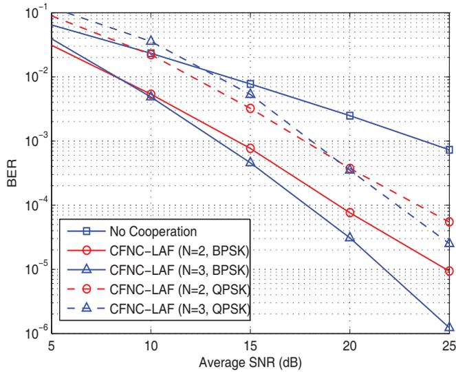
Fig. 3. BER vs. SNR (in dB) curves for CFNC-LAF with  $N = 2$  and  $N = 3$ .
