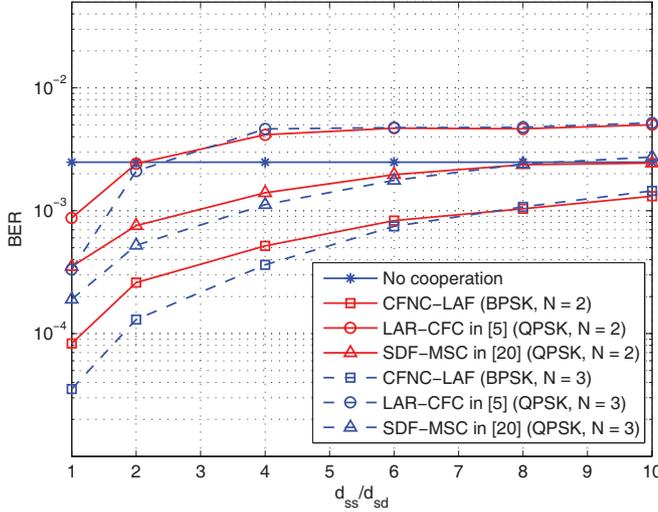
Fig. 7. BER vs. different source-destination or source-source distances for CFNC-LAF with  $N = 2, 3$  and average SNR=20dB.
