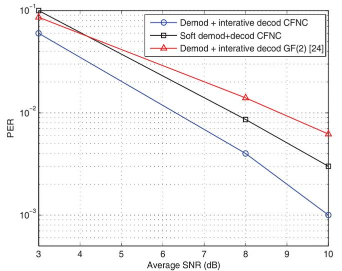
Fig. 6. PER vs. SNR (in dB) curves for the coded CFNC-LAF and bit-level network coding in [24], with  $N = 2$  and message length  $M = 100$ .
