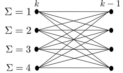
Fig. 2. Trellis diagram for  $N = 2$  and BPSK modulation ( $|\mathcal{A}_s|^N = 4$ ).
