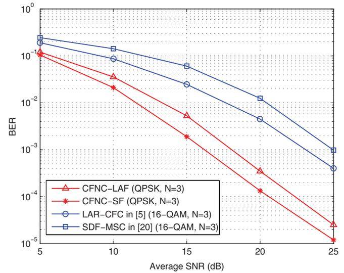
Fig. 5. BER vs. SNR (in dB) curves for CFNC-LAF and distributed space-time methods with  $N = 3$  and throughput 2 spspsu.
