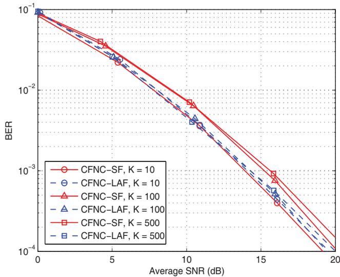
Fig. 4. BER vs. SNR (in dB) curves for the CFNC-LAF and CFNC-SF with  $N = 2$ , BPSK modulation and message length 10, 100 and 500.
