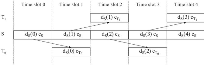
Fig. 2.  $T_0$  repeats the even frames in odd time slots while  $T_1$  repeats the odd frames in even time slots.
