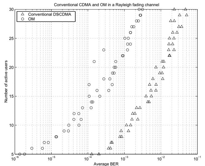
Fig. 5. Conventional DS-CDMA system and its OM counterpart. At  $PEP = 10^{-1}$  user capacity is doubled (BPSK spreading modulator with spreading gain  $K = 32$ ,  $SNR := P/\eta = 0\text{db}$ ).
