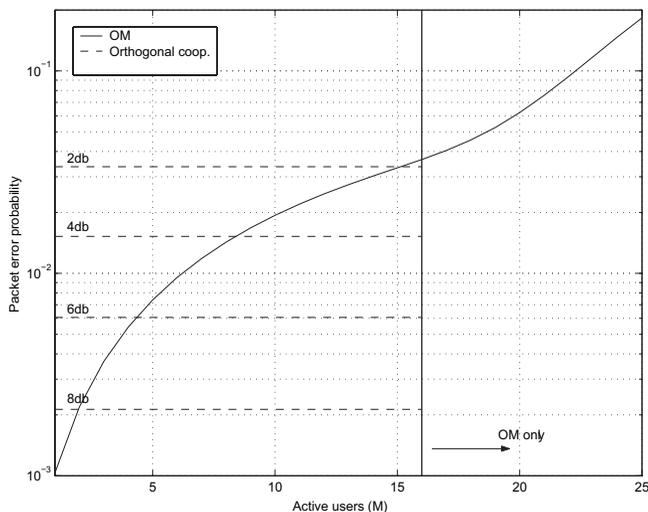
Fig. 6. Comparison of single-code OM (with diversity 2) against modified cooperative protocols using orthogonal channels (with diversity 3), both involving two cooperators per source.
