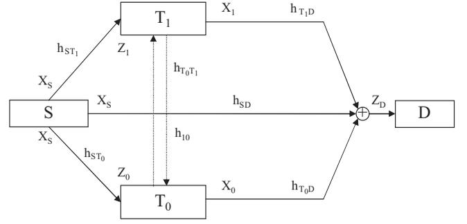
Fig. 1. Terminals  $T_0$  and  $T_1$  take turns in cooperating with  $S$ .
