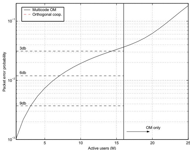
Fig. 7. Comparison of multi-code OM (with diversity 2) against modified cooperative protocols using orthogonal channels (with diversity 2), both involving one cooperator per source.
