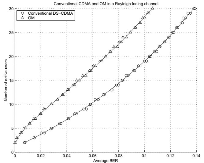
Fig. 4. Conventional DS-CDMA system and its OM counterpart (continuous lines are theoretical results, triangles and circles are simulated values). The user capacity increase is significant (BPSK spreading modulator with spreading gain  $K = 64$ ; continuous lines are theoretical results, triangles and circles are simulated values).
