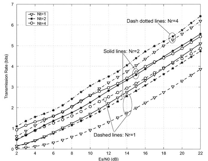
Fig. 11. The transmission rate with the desired prediction accuracy.
