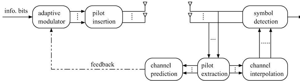
Fig. 1. The transceiver diagram.
