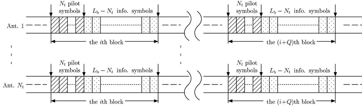
Fig. 2. The PSAM structure for multiantenna transmissions.
