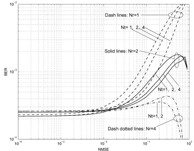
Fig. 6. BER performance at  $E_s/N_0 = 10$  dB.
