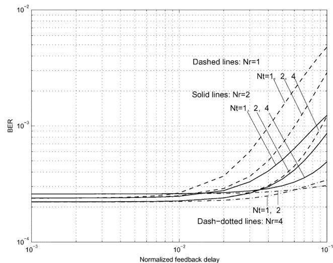
Fig. 5. Noiseless delayed feedback.
