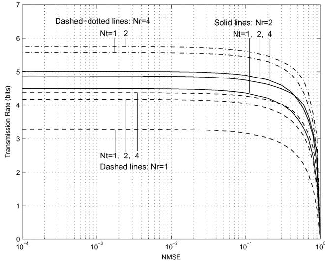
Fig. 9. Transmission rate at  $E_s/N_0 = 20$  dB.
