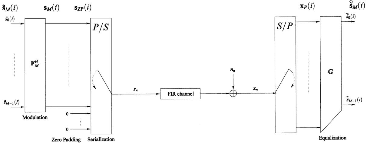
Fig. 2. Discrete model of a ZP-OFDM transceiver.
