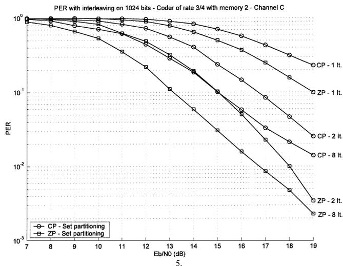
Fig. 3. CP- and ZP-OFDM with iterative decoding.
