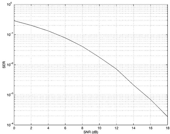
Fig. 8. SER for the MMSE equalizer (stat. meth.)
