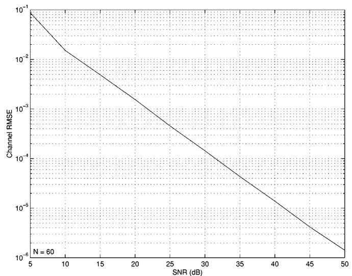
Fig. 11. Channel RMSE versus SNR (det. meth. II).
