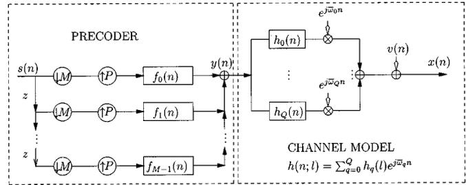
Fig. 2. Precoder and TV channel model.
