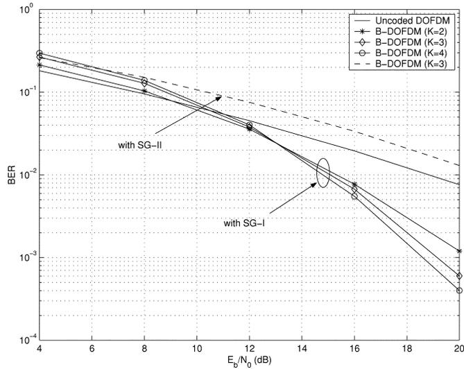
Fig. 1. B-DOFDM versus uncoded DOFDM ( $R = 2$ ).
