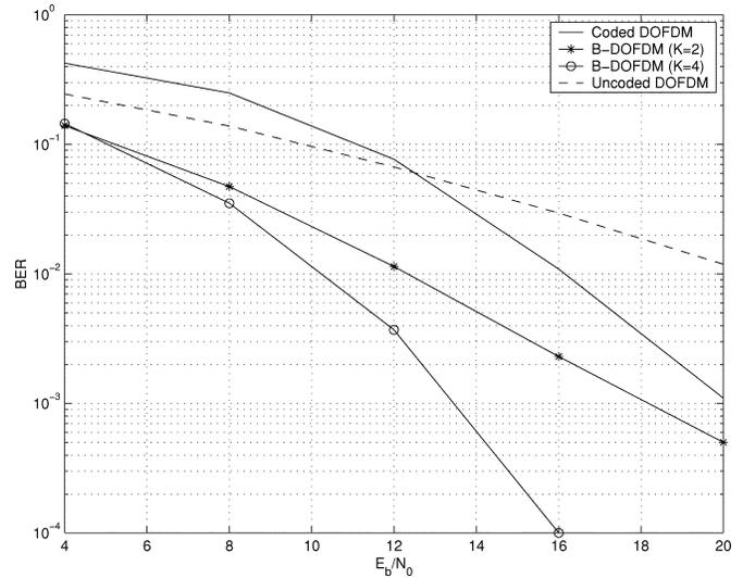
Fig. 2. B-DOFDM versus coded DOFDM ( $R = 1$ ).
