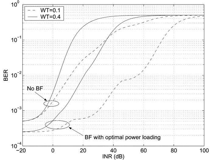
Fig. 3. BER of STBF versus INR,  $\mathcal{E}_s/N_0 = 16$  dB, channel 2.
