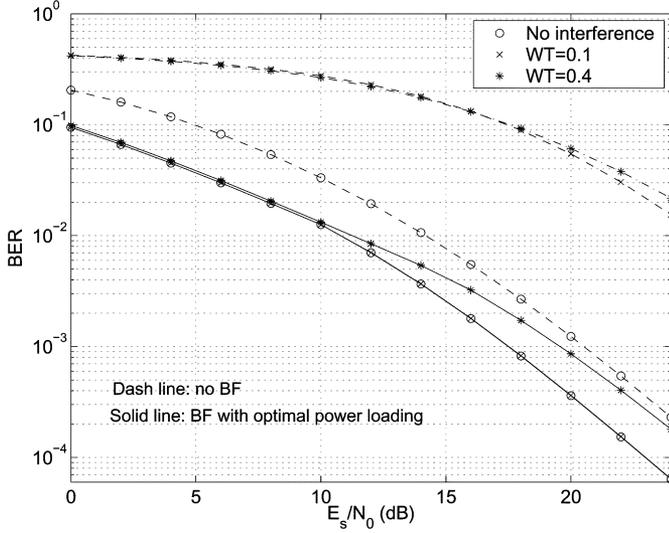
Fig. 1. BER of STBF, channel 1, INR = 10 dB.
