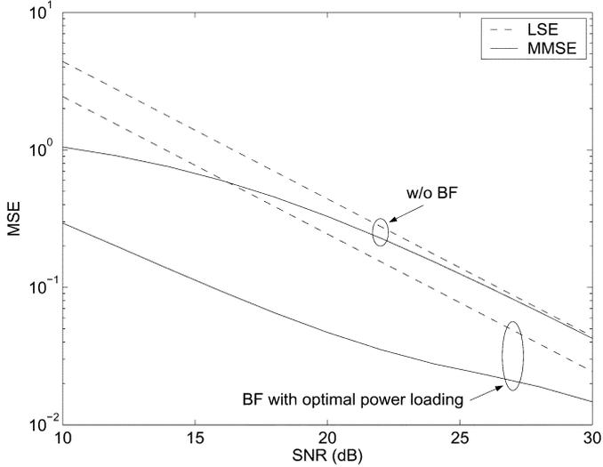
Fig. 9. MSE of channel estimators, INR = 10 dB, channel 2,  $WT = 0.1$ .
