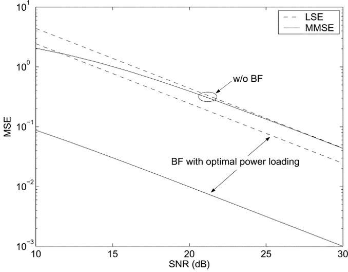
Fig. 8. MSE of channel estimators, INR = 10 dB, channel 1,  $WT = 0.1$ .
