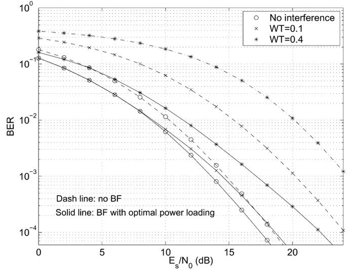
Fig. 2. BER of STBF, channel 2, INR = 10 dB.
