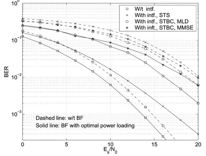
Fig. 7. Simulated BER of STBC, INR = 10 dB, channel 2,  $WT = 0.4$ .
