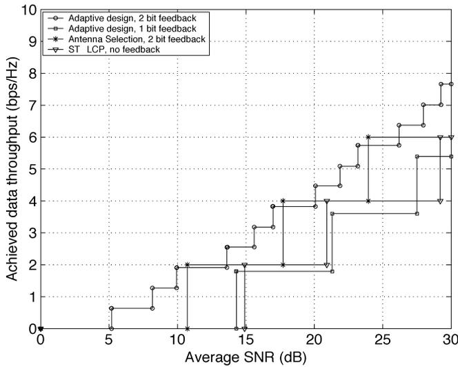
Fig. 8. Comparison with existing schemes,  $N_t = 4$ .
