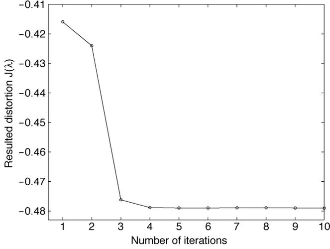
Fig. 2. Convergence of the iterative descent algorithm.
