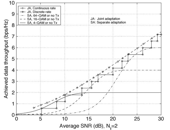
Fig. 9. Comparison with separate adaptations,  $N_t = 2$ ,  $B = 2$ .
