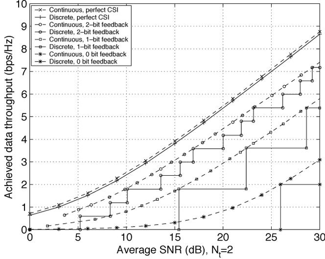
Fig. 4. Achievable data throughput,  $N_t = 2$ .  $\beta = 4.0$ ,  $\rho_0 = 0.33$  (1 b),  $\beta = 1.90$ ,  $\rho_0 = 0.66$  (2 b, average SNR  $\geq 10$  dB),  $\beta = 1.94$ ,  $\rho_0 = 0.66$  (2 b, average SNR  $< 10$  dB).
