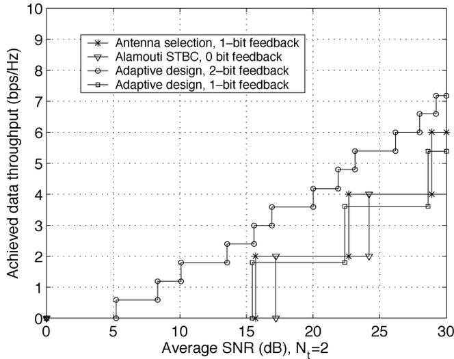
Fig. 7. Comparison with existing schemes,  $N_t = 2$ .
