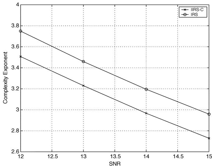
Fig. 5. Complexity exponent comparison between IIRS-C and IRS for  $M = 64$  and 2-PAM constellation.
