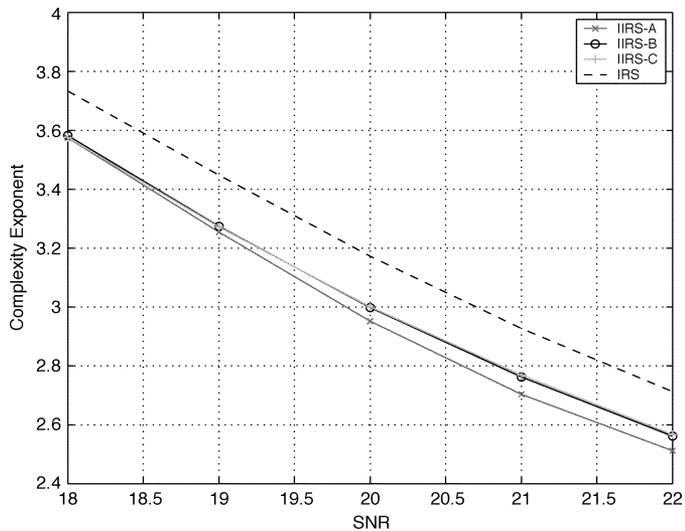
Fig. 3. Comparison of the average number of flops per decoding, in terms of complexity exponents between IIRS algorithms and the conventional IRS, for  $M = N = 32$  and 4-PAM constellation.
