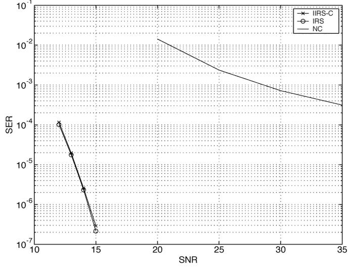
Fig. 4. SER comparison between IIRS-C, IRS, and NC for  $M = N = 64$  and 2-PAM constellation.
