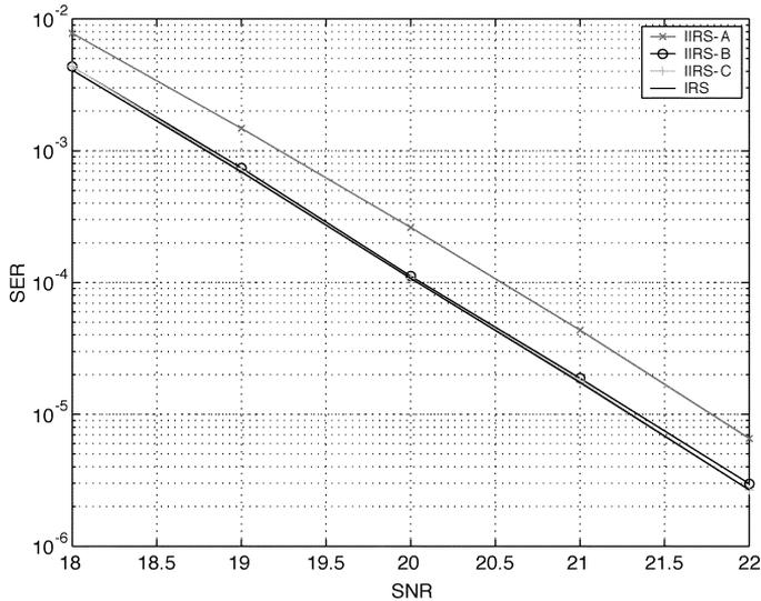
Fig. 2. SER comparison between IIRS algorithms and the conventional IRS for  $M = N = 32$  and 4-PAM constellation.
