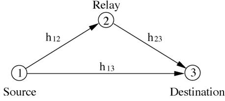
Fig. 1. System model of relayed transmissions.
