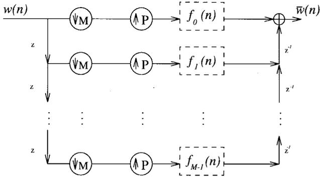
Fig. 2. Multirate encoder (analysis filterbank).
