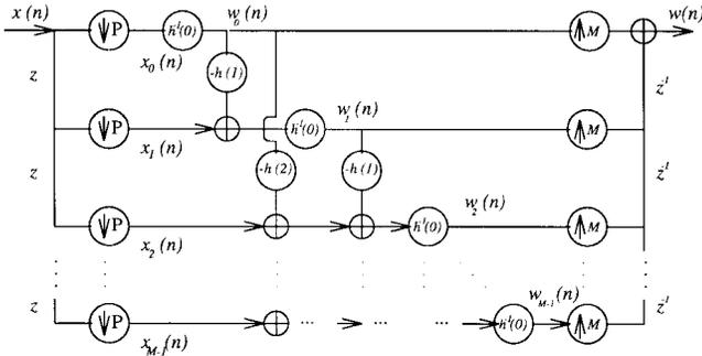
Fig. 3. Multirate decoder (synthesis filterbank).
