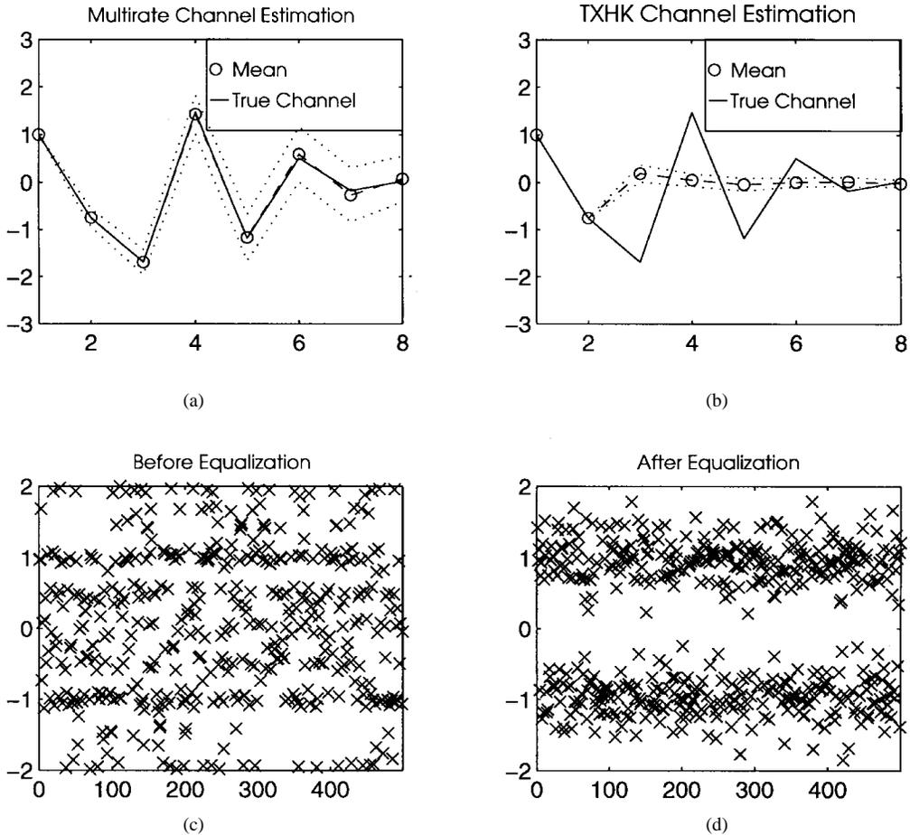
Fig. 4. (a) Channel estimation (mean  $\pm$  std) via (6). (b) Channel estimation using the method in [4]. (c) BPSK constellation before equalization and (d) after equalization.
