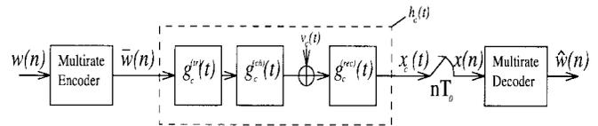
Fig. 1. Multirate transmitter-channel-receiver structure.
