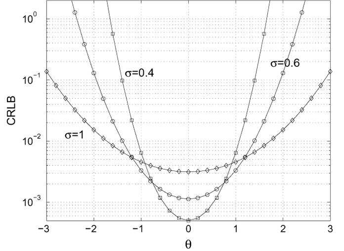
Fig. 2. CRLB versus  $\theta$  for a DES with sign detectors under i.i.d. Gaussian noise.
