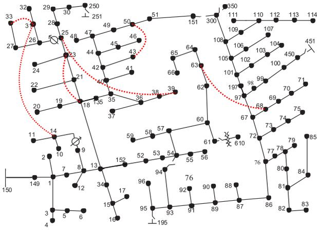
Fig. 1. IEEE 123-node distribution feeder with PV systems assumed to be present at nodes: 2, 4, 6, 10, 11, 12, 16, 17, 19, 20, 22, 24, 27, 32, 33, 36, 37, 38, 39, 41, 43, 46, 48, 49, 50, 51, 56, 59, 65, 66, 71, 75, 79, 83, 85, 88, 90, 92, 94, 96, 104, 107, 111, 114, 151, 250, 300, 450. Lines in dashed red indicate the modified meshed network that is also utilized in the case studies.
