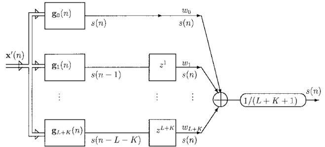
Fig. 3. Multishift equalizer and averaged input recovery.
