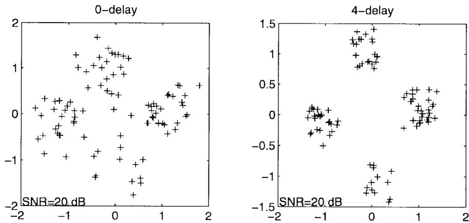
Fig. 5. Eye diagrams for different delay equalizers.
