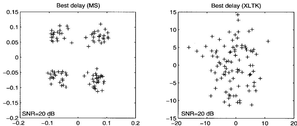
Fig. 6. Eye diagrams for MS and XLTK.
