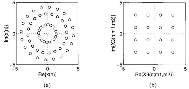
Fig. 7. Sixteen-QAM. (a) Received uncoded signal ( $\text{SNR} = \infty$ ). (b) Third-order ml-HIM ( $\text{SNR} = \infty$ ).
