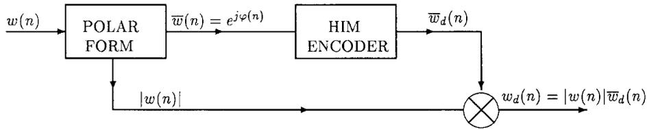
Fig. 6. Differential encoder for nonconstant modulus constellations.
