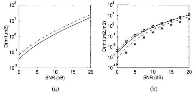
Fig. 4. Deflection versus SNR of (a) third-order ml-HIM for  $m_1 = m_2$  (solid line) and  $m_1 < m_2$  (dashed line). (b) Fourth-order ml-HIM for  $(m_1, m_2, m_3) = (1, 1, 1)$  (stars),  $(1, 1, 2)$  (dashed line),  $(1, 2, 4)$  (dash-dotted line),  $(2, 3, 4)$  (circles),  $(1, 2, 3)$  (solid line), and  $(1, 4, 8)$  (x-marks).
