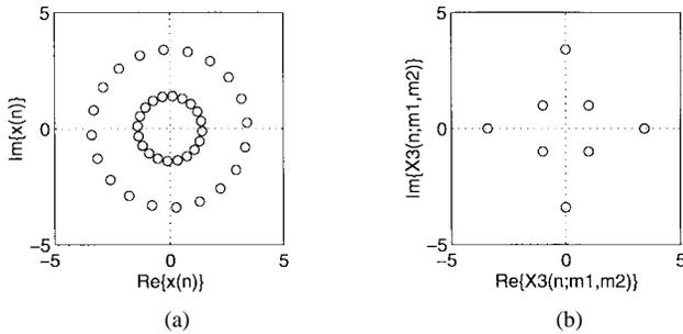
Fig. 9. Eight AM-PM. (a) Received uncoded signal ( $\text{SNR} = \infty$ ). (b) Third-order ml-HIM ( $\text{SNR} = \infty$ ).
