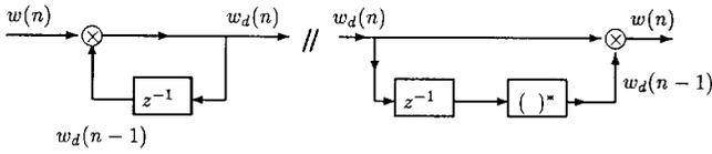
Fig. 2. First-order differential encoder/decoder ( $m_1 = 1$ ).
