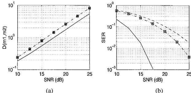
Fig. 11. Sixteen-QAM. (a) Deflection of third-order ml-HIM versus SNR for  $(m_1, m_2) = (1, 1)$  (solid line),  $(1, 2)$  (dash-dotted line),  $(1, 3)$  (circles),  $(1, 4)$  (stars). (b) SER versus SNR with third-order ml-HIM decoder for  $(m_1, m_2) = (1, 1)$  (dashed line),  $(1, 2)$  (dash-dotted line),  $(1, 3)$  (circles), and  $(1, 4)$  (x-marks). The solid line in (b) denotes the SER of an ideal 16-QAM ( $\theta_c(t) = 0$ ).
