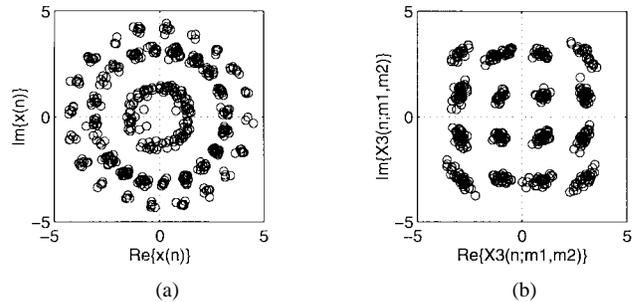
Fig. 8. Sixteen-QAM. (a) Received uncoded signal ( $\text{SNR} = 25$  dB). (b) Third-order ml-HIM ( $\text{SNR} = 25$  dB).
