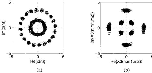
Fig. 10. Eight AM-PM. (a) Received uncoded signal ( $\text{SNR} = 25$  dB). (b) Third-order ml-HIM ( $\text{SNR} = 25$  dB).
