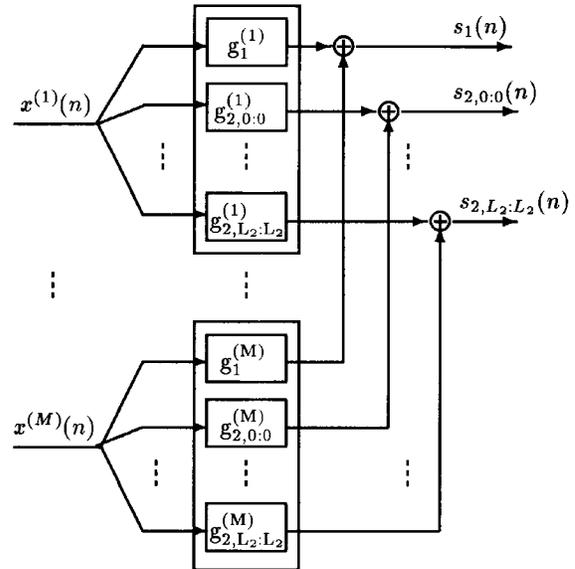
Fig. 3. Structure of the deconvolver ( $P = 2$ ).
