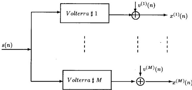
Fig. 1. SIMO nonlinear Volterra channel.
