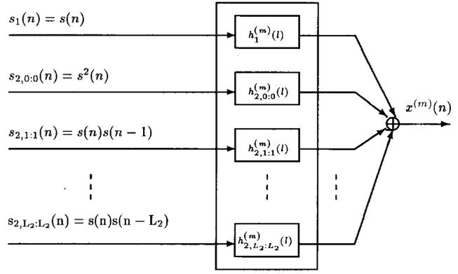
Fig. 2. Structure of the  $m$ th subchannel ( $P = 2$ ).
