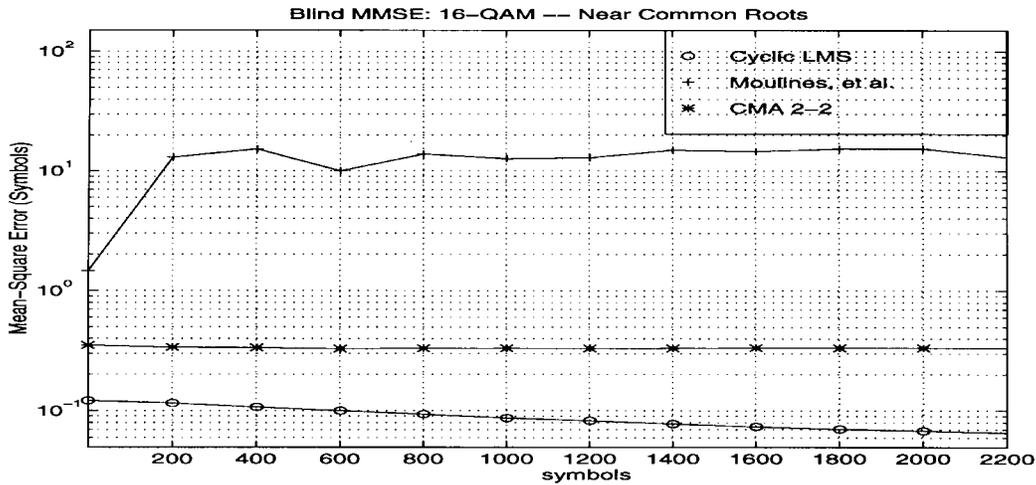
Fig. 11. Mean-square symbol error: Comparison at SNR = 30 dB.
