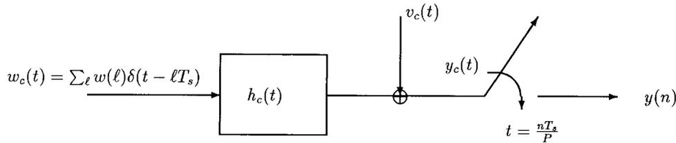
Fig. 1. Fractionally sampled communication system.
