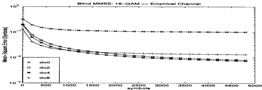
Fig. 9. Comparison of MSE for delays  $d$ : Cyclic RLS at SNR = 30 dB.
