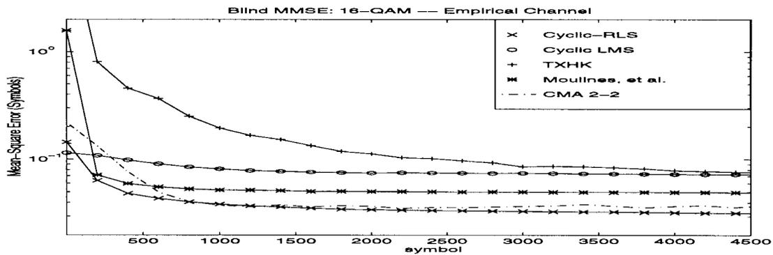
Fig. 8. Mean-square symbol error: Comparison at SNR = 30 dB.
