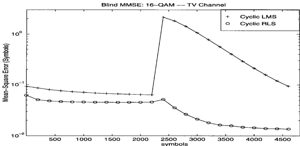
Fig. 13. Mean-square symbol error: Time-varying channel at SNR = 20 dB.
