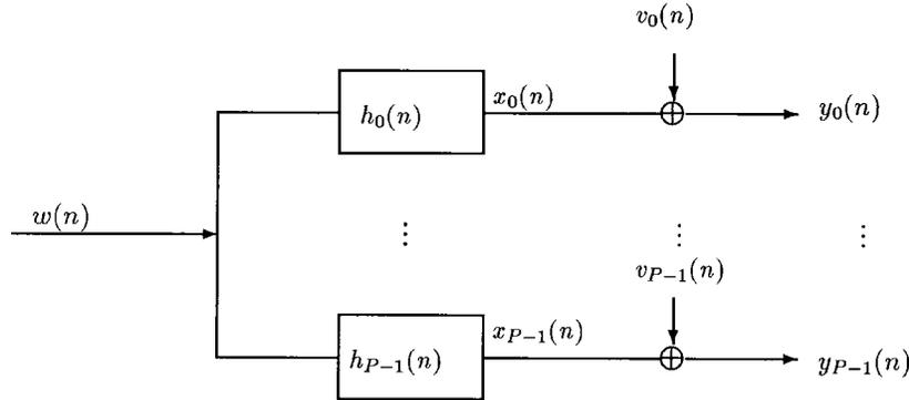
Fig. 2. Multichannel model for FS channel.
