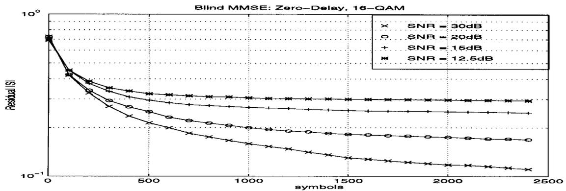
Fig. 6. Residual ISI: Direct MMSE.
