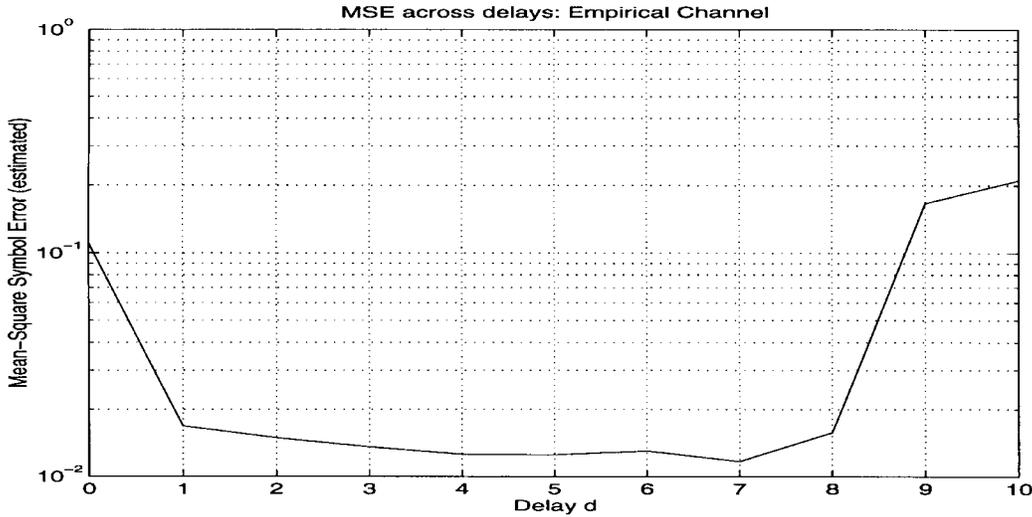
Fig. 14. Selection of optimum delay: Empirical channel.
