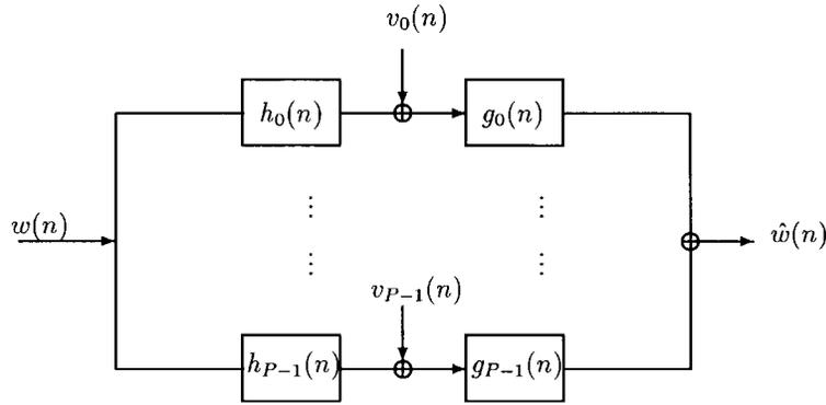
Fig. 3. Linear equalization for FS channels.
