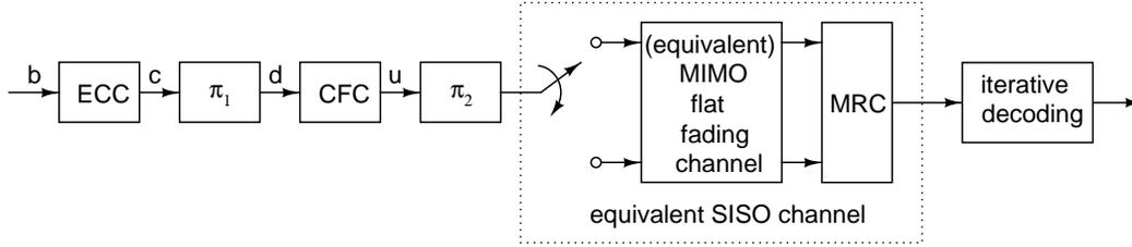
Figure 1: Joint GF and CF coded ST system Model
