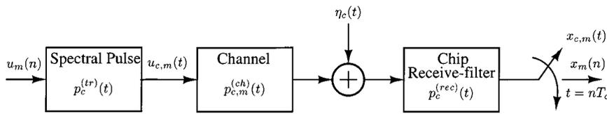
Fig. 2. Baseband continuous-time model for user  $m$ , sampled at the chip rate;  $p_c^{(tr)}(t)$ ,  $p_c^{(ch)}(t)$ ,  $p_c^{(rec)}(t)$  denote, respectively, the transmit-chip waveform, the  $m$ th user's channel, and the receive-chip waveform.
