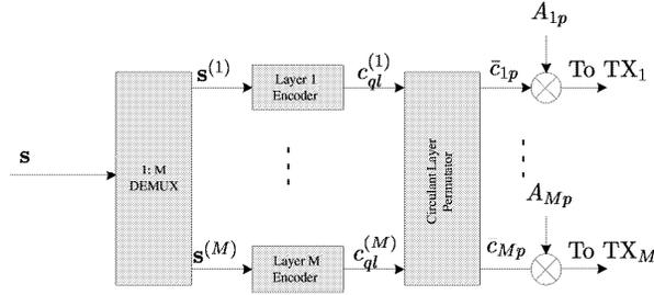
Fig. 1. Layered space-time encoder
