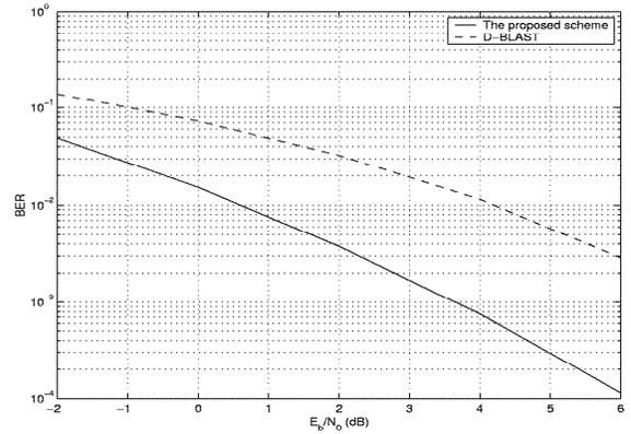
Fig. 3. Performance comparison with D-BLAST
