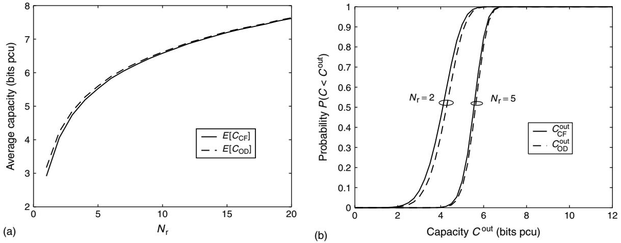
Fig. 12. Comparisons of \$C\_{CF}\$ and \$C\_{OD}\$ when \$N\_t = 2\$.
