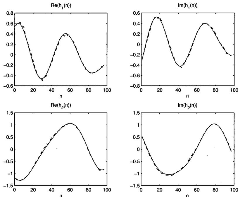
Fig. 3. True (solid curves) and KF-based estimate (dashed curves) of channel variations.
