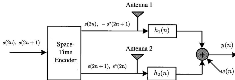
Fig. 1. Discrete time equivalent baseband model.
