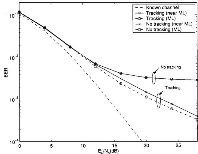
Fig. 2. BER improvement with KF-based channel tracking (the BER curve of no channel tracking with ML decoding overlaps that with near-ML decoding).
