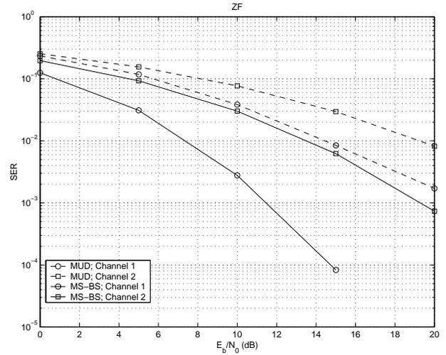
Fig. 3.  $SER$  vs.  $E_b/N_0$  for ZF receiver for binary symbols with  $N_f = 3$ ,  $N_c = 8$ , and  $K = 2$ .
