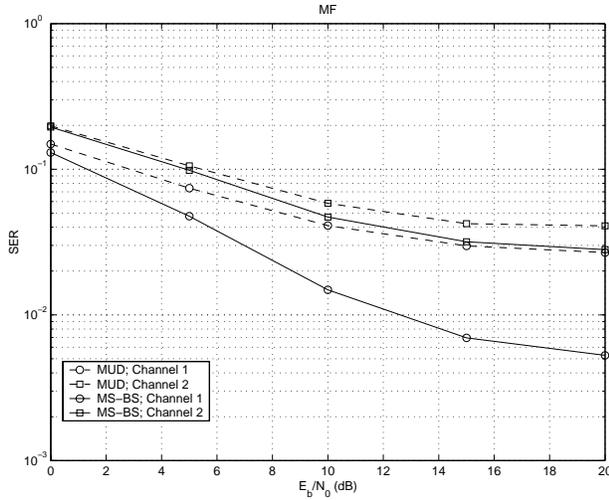
Fig. 2.  $SER$  vs.  $E_b/N_0$  for MF receiver for binary symbols with  $N_f = 3$ ,  $N_c = 8$ , and  $K = 2$ .
