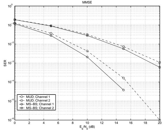
Fig. 4.  $SER$  vs.  $E_b/N_0$  for MMSE receiver for binary symbols with  $N_f = 3$ ,  $N_c = 8$ , and  $K = 2$ .
