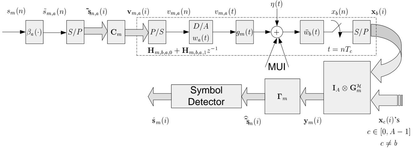
Fig. 1. Continuous and discrete-time equivalent system model of the  $m$ -th user (only the  $a$ -th branch at the transmitter and the  $b$ -th branch at the receiver are shown).
