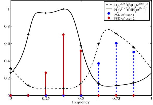
Fig. 2. Optimal transmit-PSDs and ratios of channel transfer function gains
