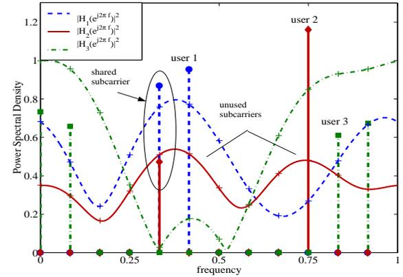
Fig. 3. Optimal transmit-PSDs along with  $|H_1(e^{j2\pi f})|^2$ ,  $|H_2(e^{j2\pi f})|^2$ , and  $|H_3(e^{j2\pi f})|^2$
