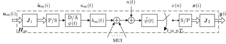
Fig. 1. Continuous and discrete-time baseband equivalent multichannel model.
