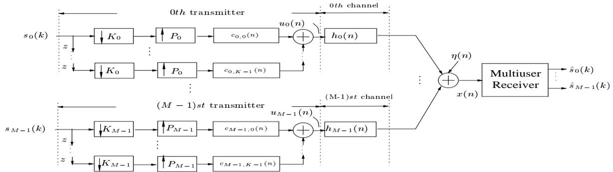
Figure 1: Multi-rate block-spread CDMA system
