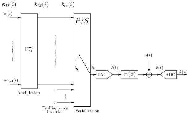
Figure 1: Discrete model of the TZ precoder
