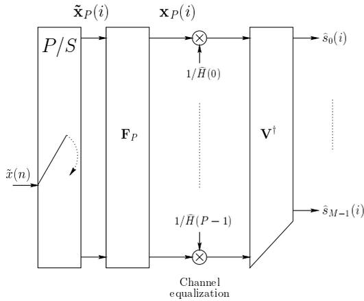
Figure 2: TZ-OFDM-FAST Equalizer
