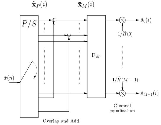
Figure 3: OLA equalization scheme
