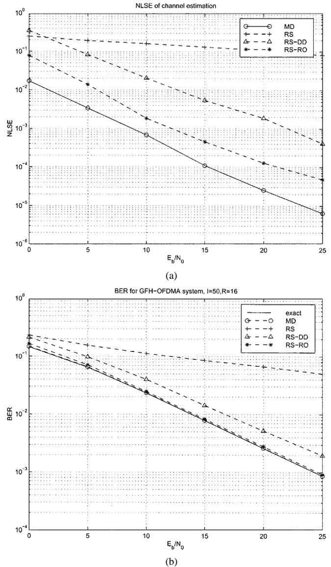
Fig. 6. Blind channel estimation (QPSK). (a) Channel NLSE. (b) BER.
