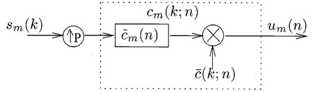
Fig. 2. The  $m$ th user's structured long code transmission model.
