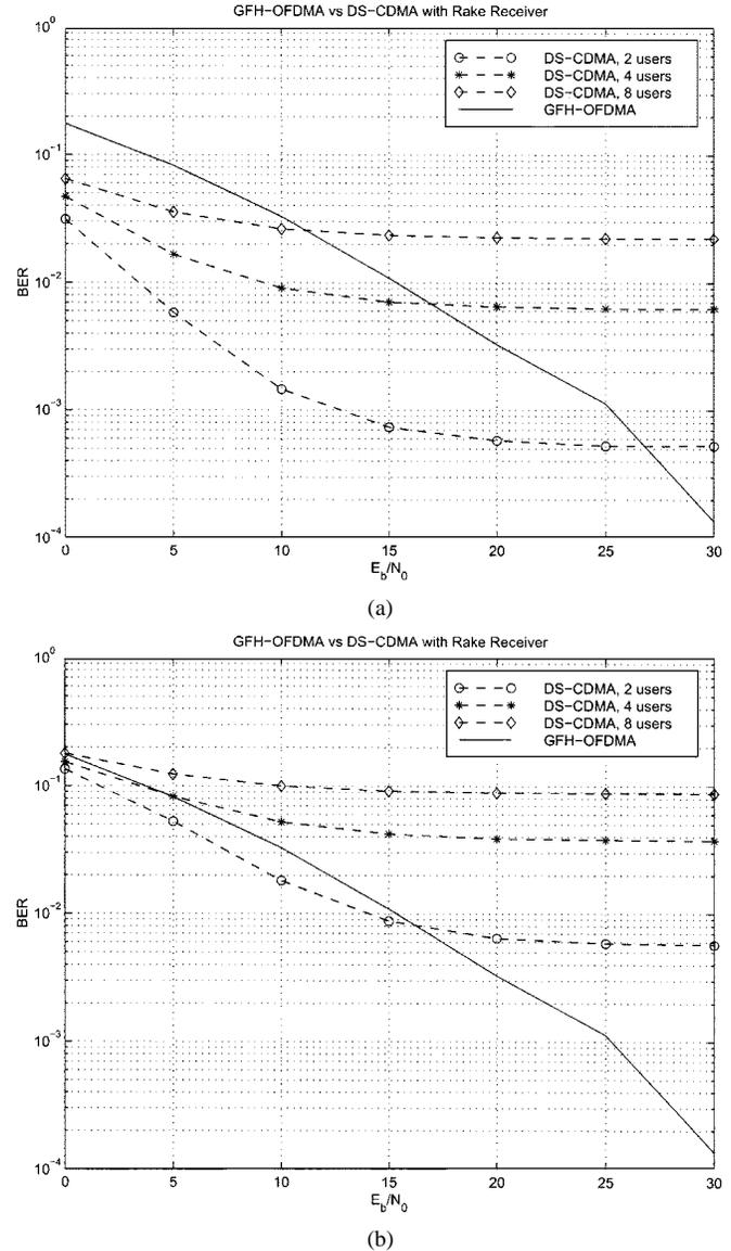
Fig. 4. Comparisons of GFH-OFDMA with long code DS-CDMA. (a) OFDM codes. (b) W-H codes.
