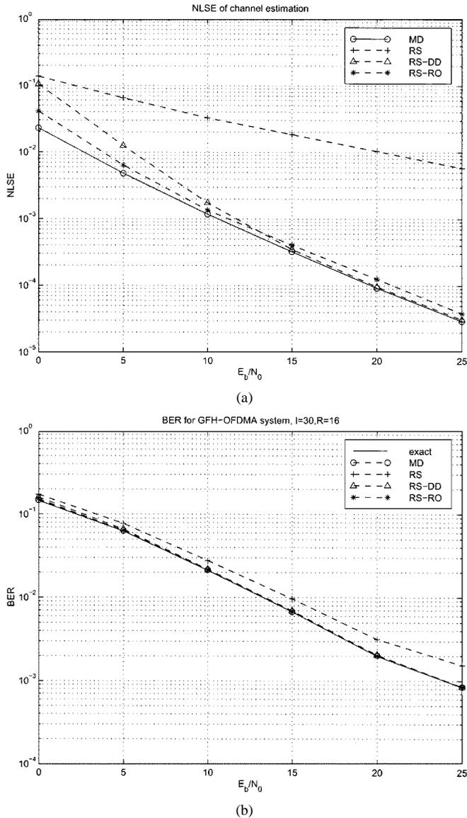
Fig. 5. Blind channel estimation (BPSK). (a) Channel NLSE. (b) BER.
