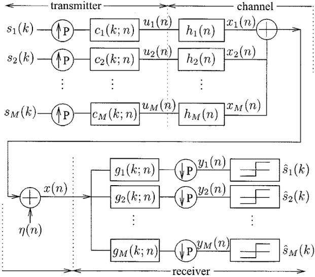
Fig. 1. Discrete-time baseband long code CDMA system.
