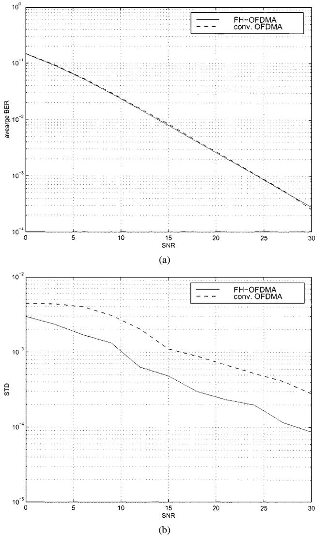
Fig. 3. Comparisons of FH-OFDMA with conventional OFDMA. (a) Mean BER. (b) STD BER.
