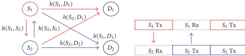
FIGURE 1: Source terminals  $S_1$  and  $S_2$  cooperate in transmitting to their respective destinations  $D_1$  and  $D_2$  by creating a distributed virtual antenna array (VAA).
