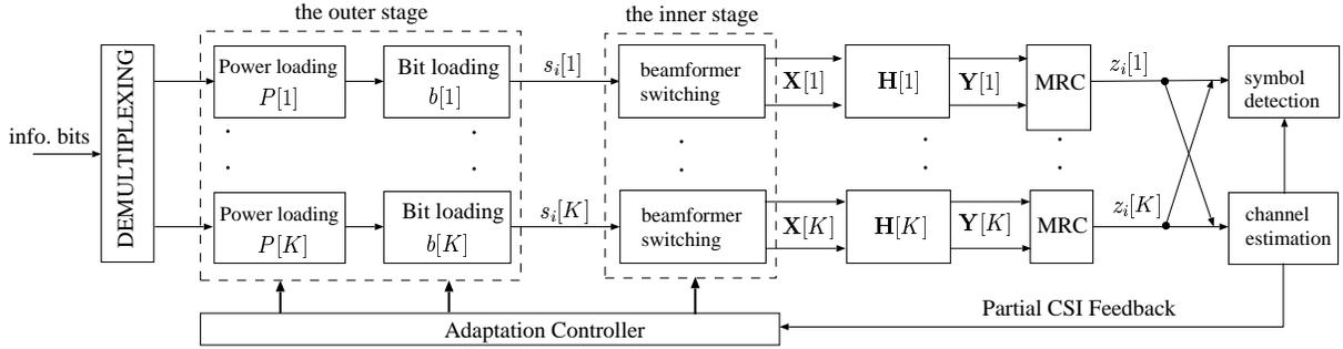
Figure 1: Discrete time baseband equivalent system model
