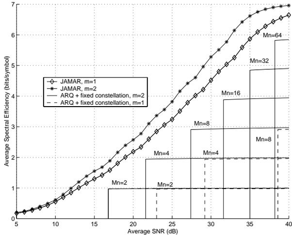
Figure 2: Average spectral efficiency vs.  $\bar{\gamma}$
