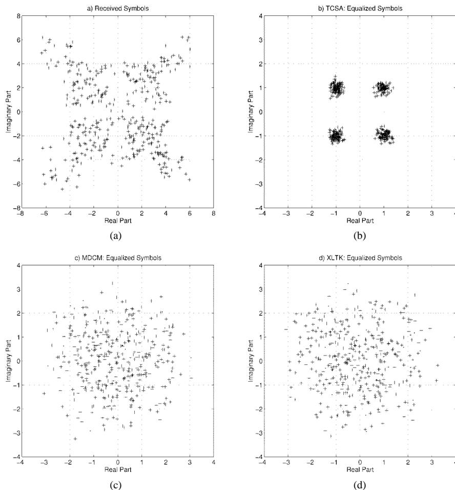
Fig. 10. Received symbols. Before and after equalization.
