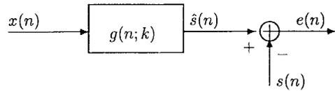
Fig. 4. Cyclic Wiener filtering.
