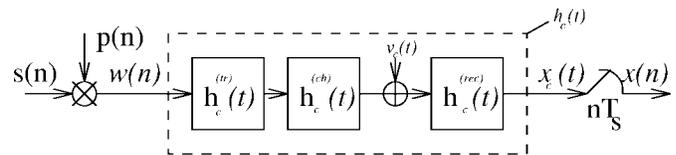
Fig. 1. Baseband transmission channel.
