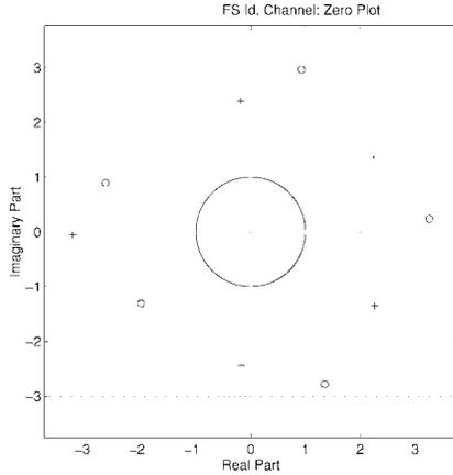
Fig. 16. FS identifiable channel. Zero plots of subchannels.
