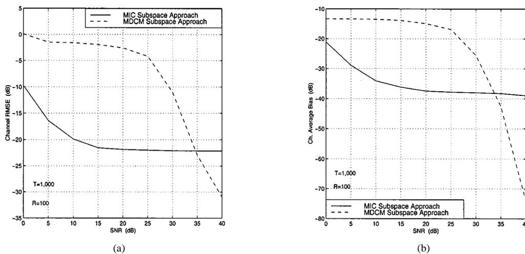
Fig. 12. Identifiability limit. Channel average RMSE/Bias versus SNR.
