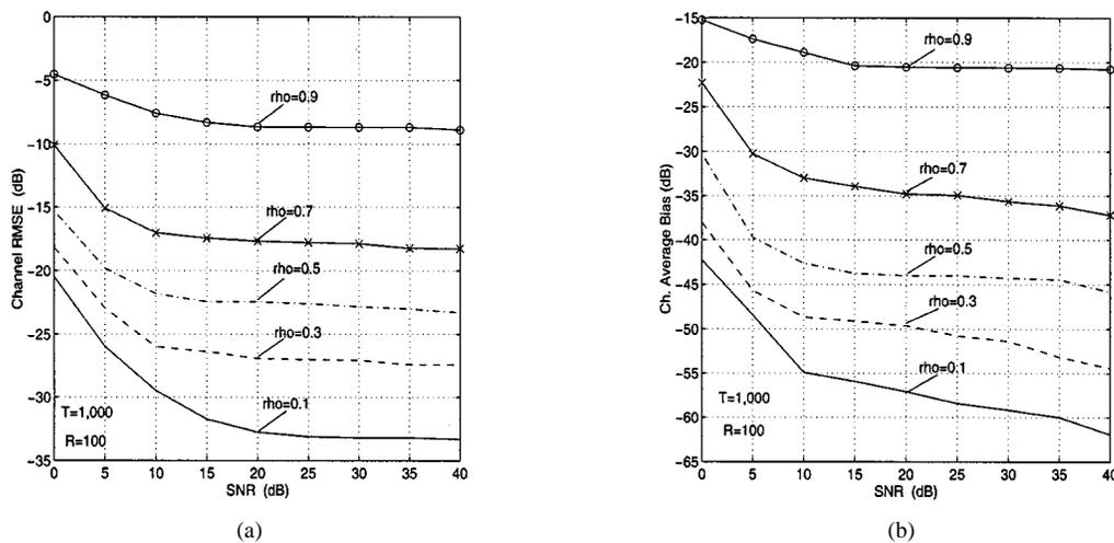
Fig. 10. Channel average RMSE/Bias versus SNR. Comparisons.
