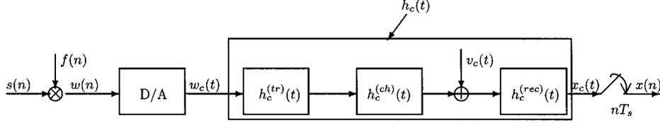
Fig. 1. Baseband transmission channel.
