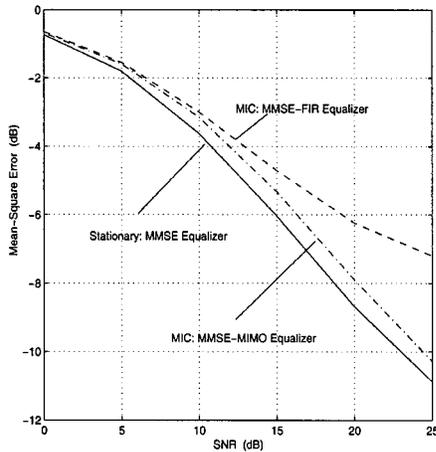
Fig. 5. MMSE linear equalization. MSE comparisons.
