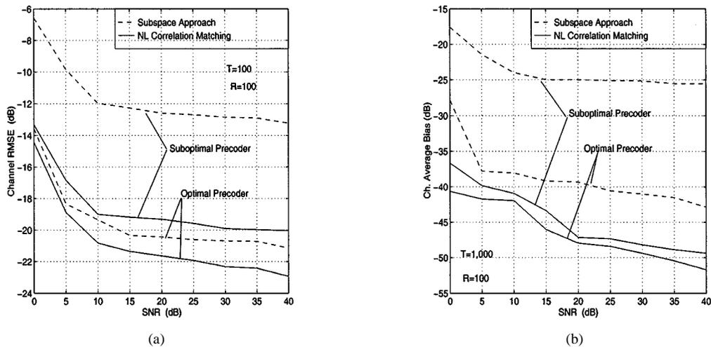
Fig. 9. Channel average RMSE/Bias versus SNR.
