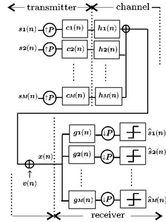
Fig. 1. Multirate discrete-time CDMA model.
