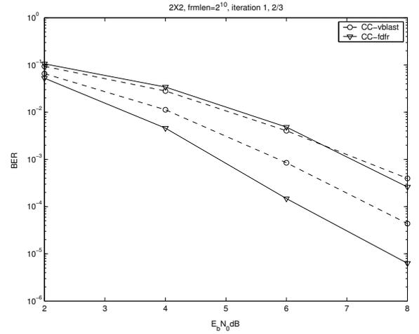
Fig. 2. 1/2 convolutional codes with FDFR v.s. 1/2 convolutional codes with V-BLAST in  $2 \times 2$  setup
