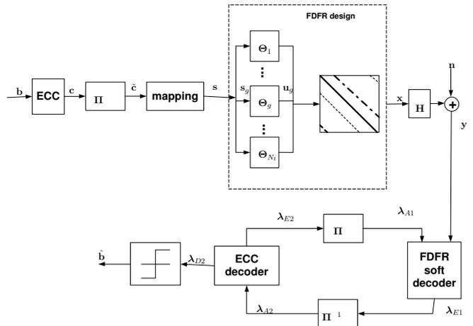
Fig. 1. the coded FDFR system model
