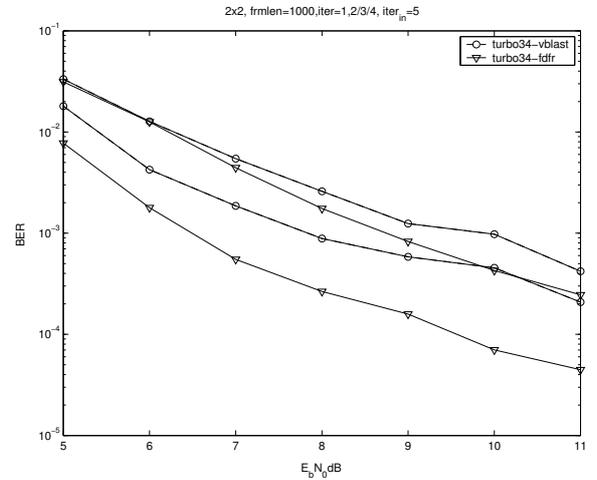
Fig. 3. 3/4 turbo codes with FDFR v.s. 3/4 turbo codes with V-BLAST in  $2 \times 2$  setup
