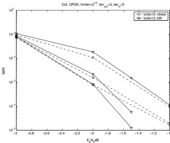
Fig. 5. 1/2 turbo codes with FDFR v.s. 1/2 turbo codes with V-BLAST in  $2 \times 5$  setup
