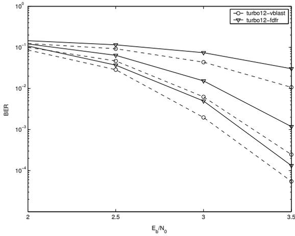
Fig. 4. 1/2 turbo codes with FDFR v.s. 1/2 turbo codes with V-BLAST in  $2 \times 2$  setup
