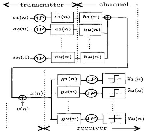
Fig. 1. Multirate discrete-time CDMA model.
