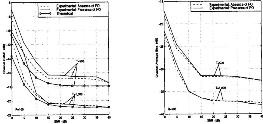
Fig. 8. Channel Avg. RMSE/bias versus SNR.
