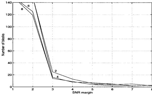
Fig. 10. Number of blocks as a function of the SNR margin  $\xi(N)$  for different number of bits.
