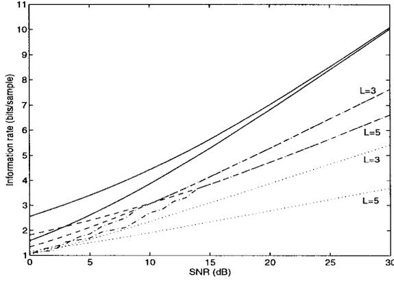
Fig. 7. Channel capacity (solid line) and information rates, in bits per sample, achieved with optimal filterbank, loading algorithm #1 (dashed-dotted line) and #2 (dashed line), and with DMT (dotted line), relative to two channels having  $L = 3$  and  $L = 5$  zeros on the unit circle ( $M = 32$ ).
