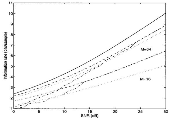
Fig. 6. Channel capacity (solid line) and information rates, in bits per sample, achieved with optimal filterbank, loading algorithm #1 (dashed-dotted line) and #2 (dashed line), and with DMT (dotted line), using two different block lengths  $M$ .
