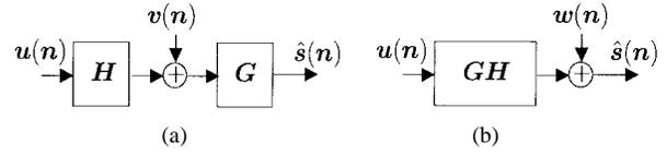
Fig. 2. Matrix equivalent model of Fig. 1.
