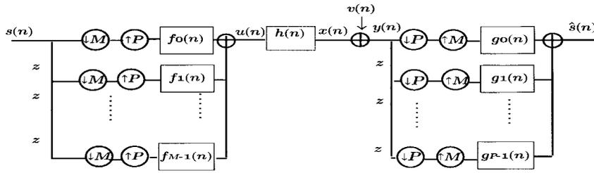
Fig. 1. Multirate discrete-time equivalent transmitter/channel/receiver model.
