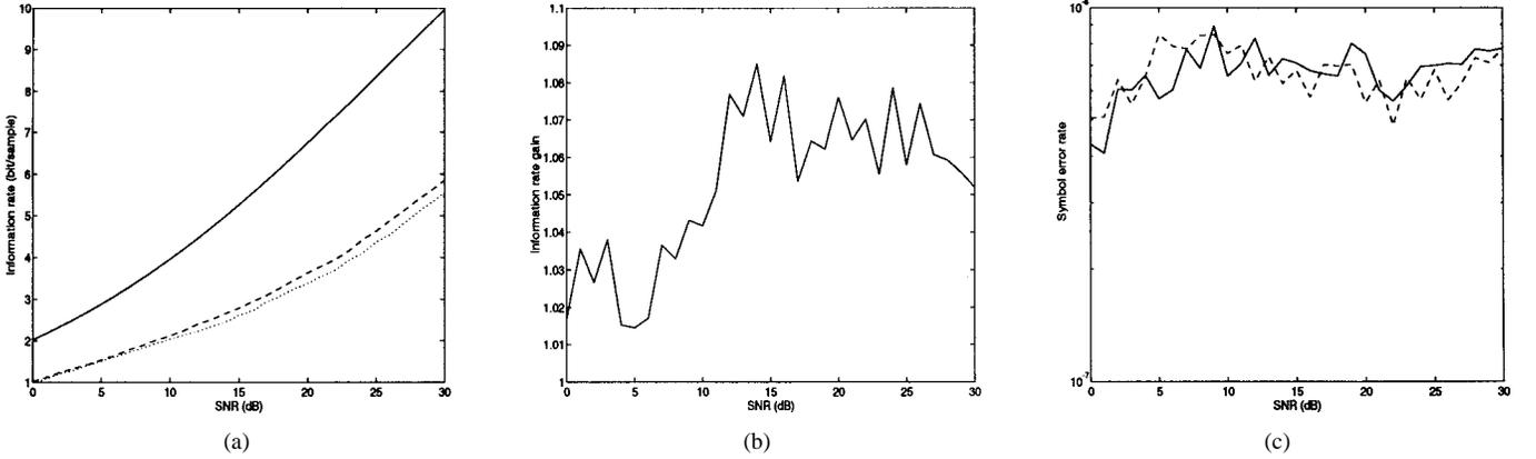
Fig. 9. Results pertaining to channel 2: (a) channel capacity (solid line) and information rates (bps) achieved with our method (dashed line) and with DMT (dotted line); (b) gain in information rate achieved with our method with respect to DMT; and (c) symbol error probability for DMT (dashed) and this paper's method (solid).
